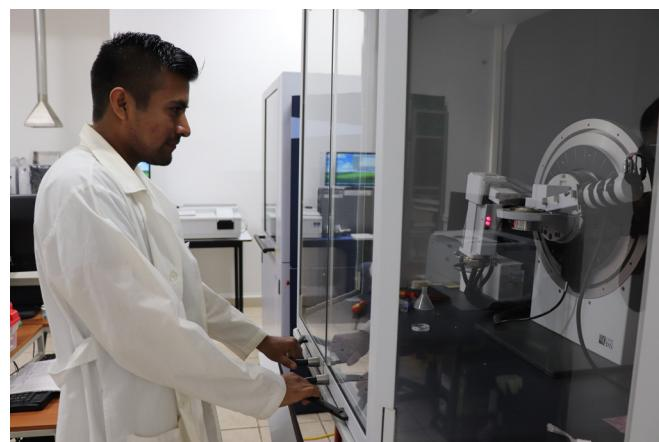
*Single crystal X-ray Diffractometer and Powder X-ray Diffractometer (left - right). Instrumental Chemistry Lab. UNPA. Tuxtepec Campus*
