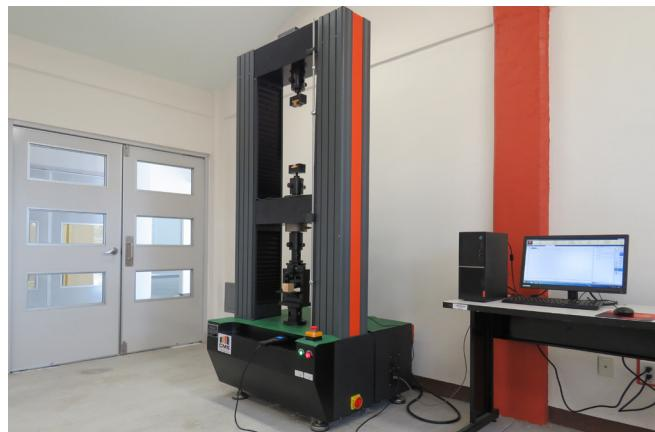
*CMS Metrology Universal Machine for Wood Mechanics Testing*
