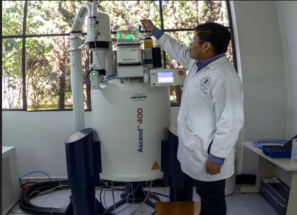
*NMR - Nuclear Magnetic Resonance Spectroscopy. UTM. Huajuapan de León.*
