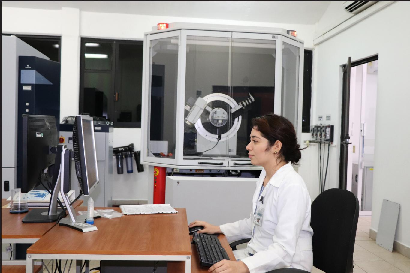
*Powder X-ray Diffractometer. Instrumental Chemistry Laboratory. University of Papaloapan. Tuxtepec Campus.*
