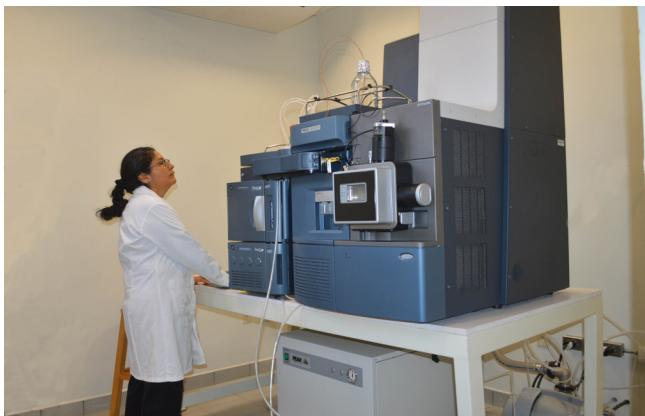
*Ultra high pressure liquid chromatography coupled to a mass spectrometer. Biotechnology Lab. UTM. Huajuapan de León*
