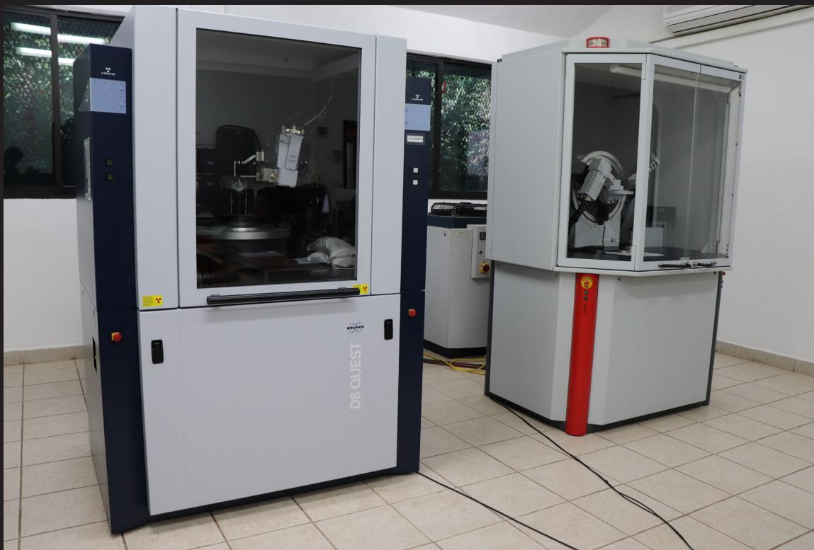
*Single Cristal X-ray Diffractometer and Powder X-ray Diffractometer.
