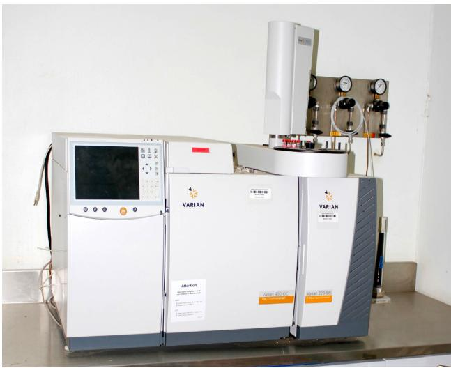
*Gas chromatography coupled to a mass spectrometer.
